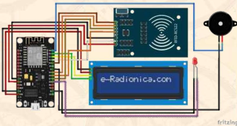
GAMBAR 6, RANGKAIAN ELEKTRONIK RFID READER
