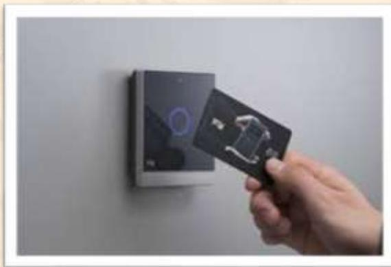
GAMBAR 1, SISTEM ABSENSI RFID
